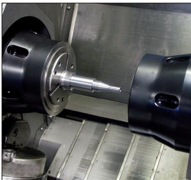
With a pullback collet chuck, closing the collet is accomplished by pulling it back into the chuck body, whereas with an Accu-Length™ chuck, the collet is rigidly fixed to the chuck body and a tapered sleeve pushes forward over the collet to compress it.
