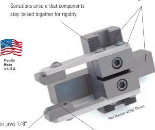
Unit is very easy to use — simply set gap between jaws 1/8" smaller than stock size. As the bar puller slides over the bar along the x-axis, the fingers flex to provide the gripping force. The turret then retracts along the z-axis, pulling the bar out to the desired position.
