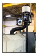
Useful for open-top machine tools such as vertical machining centers where there is no option for mounting the mist collector on top of the machine.
