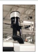
A great option when you want the mist collector off the floor, but your machine doesn't lend itself to direct mounting because the ideal intake location within the machine enclosure is not compatible with the mist collector positioning.
