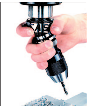
3. Removing drill chuck holder with one hand.
