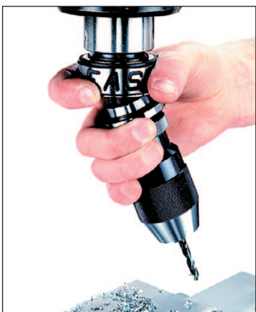
3. Removing drill chuck holder with one hand.
