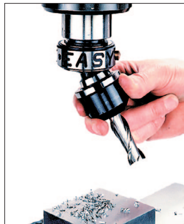
4. Inserting endmill holder and endmill for next operation.
