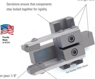
Unit is very easy to use — simply set gap between jaws 1/8" smaller than stock size. As the bar puller slides over the bar along the x-axis, the fingers flex to provide the gripping force. The turret then retracts along the z-axis, pulling the bar out to the desired position.
