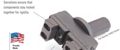
Unit is very easy to use — simply set gap between jaws 1/8" smaller than stock size. As the bar puller slides over the bar along the x-axis, the jaws compress heavy-duty internal die springs to provide high gripping force. The turret then retracts along the z-axis, pulling the bar out to the desired position.
