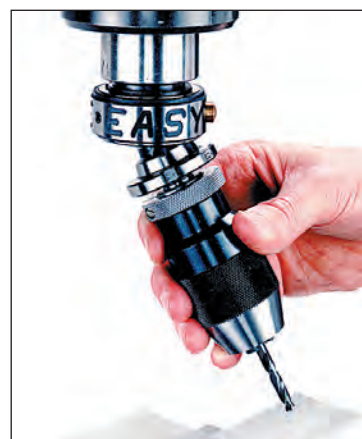
2. Loading drill chuck holder and drill into body.
