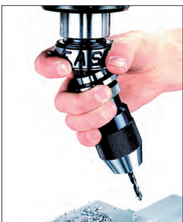
3. Removing drill chuck holder with one hand.
