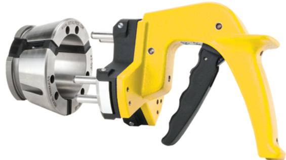
1. The unique collets are constructed of hardened steel segments securely joined together by vulcanized rubber. Each collet contains an annular hook and groove configuration on the rear section of its outer diameter.
