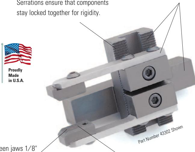
Unit is very easy to use – simply set gap between jaws  $1/8"$  smaller than stock size. As the bar puller slides over the bar along the x-axis, the fingers flex to provide the gripping force. The turret then retracts along the z-axis, pulling the bar out to the desired position.
