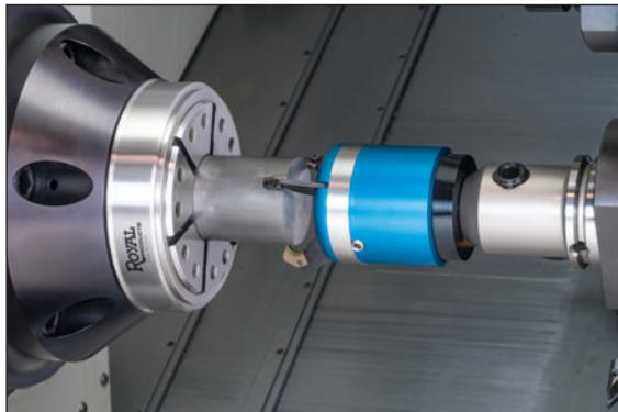
The Grippex has a wide gripping range of  $\frac{1}{8}$ " –  $3\frac{1}{8}$ ". Higher capacity gripping fingers are also available.
