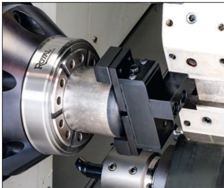
Serrations ensure that components stay locked together for rigidity.
