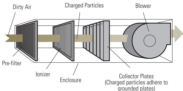
**Variable Efficiency** Although electrostatic systems are very efficient when the collection plates are clean, the efficiency drops off drastically as the plates become covered with particles. Each time a particle deposits on a plate, it eliminates a spot for other particles to adhere to.
