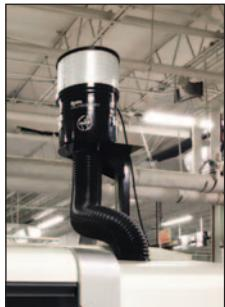
A great option when you want the mist collector off the floor, but your machine doesn't lend itself to direct mounting because the ideal intake location within the machine enclosure is not compatible with the mist collector positioning.
