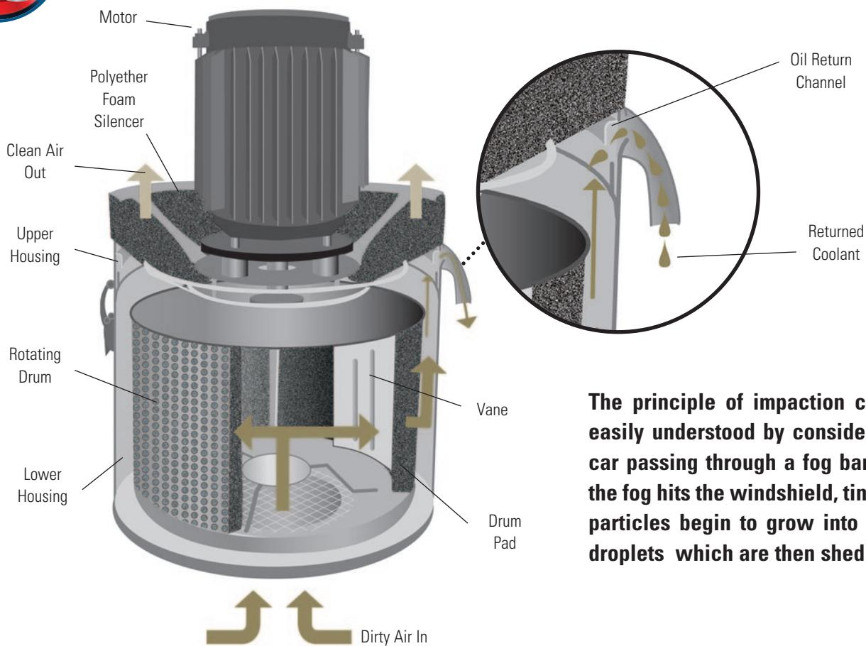
**The principle of impaction can be easily understood by considering a car passing through a fog bank. As the fog hits the windshield, tiny mist particles begin to grow into water droplets which are then shed off.**
