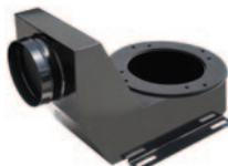
The key to this system is the Royal Plenum, which has been optimized for minimal cfm loss. The plenum also functions as a coarse pre-filter by forcing fines and chips to drop out of the mist stream due to the internal airflow directional change.
