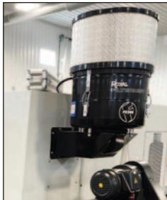
The side mount bracket is specifically designed for models FX-300 and 575. It mounts directly to the side of the machine tool with no ducting required.
