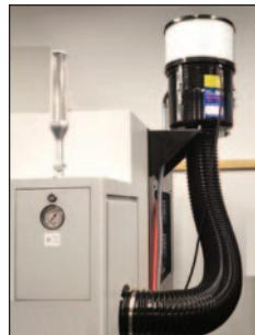
Wall mount brackets are available for all models. These brackets can be mounted to walls or I-beams, and can also be used to mount the mist collector to the side of the machine tool as shown.
