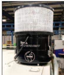
Very cost-effective and **our most popular mounting method**. The mist collector mounts to the top of the machine tool enclosure directly over the appropriate intake position.
