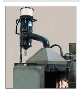
Grinding applications can sometimes be more demanding than typical turning and milling applications because grinding produces fine dust particles that become entrained in the mist stream. Over time, this dust can accumulate on the drum pads, resulting in the need for more frequent maintenance. If regular maintenance is not performed and a significant volume of solid matter builds up in the drum, balance and vibration issues may arise.
