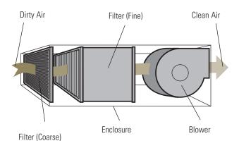
**High Operating Costs** The biggest drawback of media-type filtration systems is the high operating cost associated with replacement filters. These filters are designed to retain contaminants, so they will become clogged with use. Usually they are made from media that cannot be cleaned, so the only alternative is replacement. Depending upon the cost of the filters and the replacement frequency, this type of system can be quite expensive to operate over the long term.
