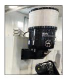
The side mount bracket is specifically designed for models FX-300 and 575. It mounts directly to the side of the machine tool with no ducting required.
