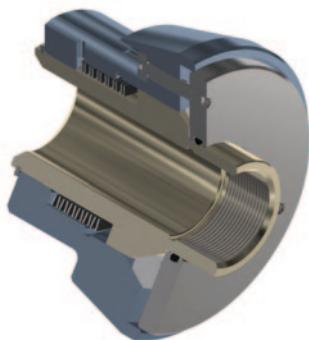
To maintain precise z-axis positioning of the workpiece, the collet in a Royal Accu-Length™ Collet Chuck is fixed to the body and the chuck's closing sleeve pushes forward over the collet to compress it. The collet, and therefore the workpiece, remains fixed in the z-position.
