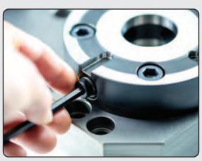
A few turns of a hex key and you're locked in and ready to machine. **Simple manual actuation** makes Z-Lock<sup>TM</sup> a breeze to implement.
