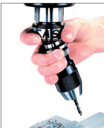
3. Removing drill chuck holder with one hand.
