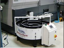
The Royal Rota-Rack® is an automatic accumulator that can be used with any bar-fed CNC lathe to safely collect finished parts, providing hours of highly profitable, unmanned production.
